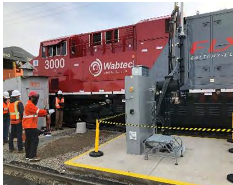
Figure 3 Image of BEL While Charging at the BNSF Stockton Mormon Yard
