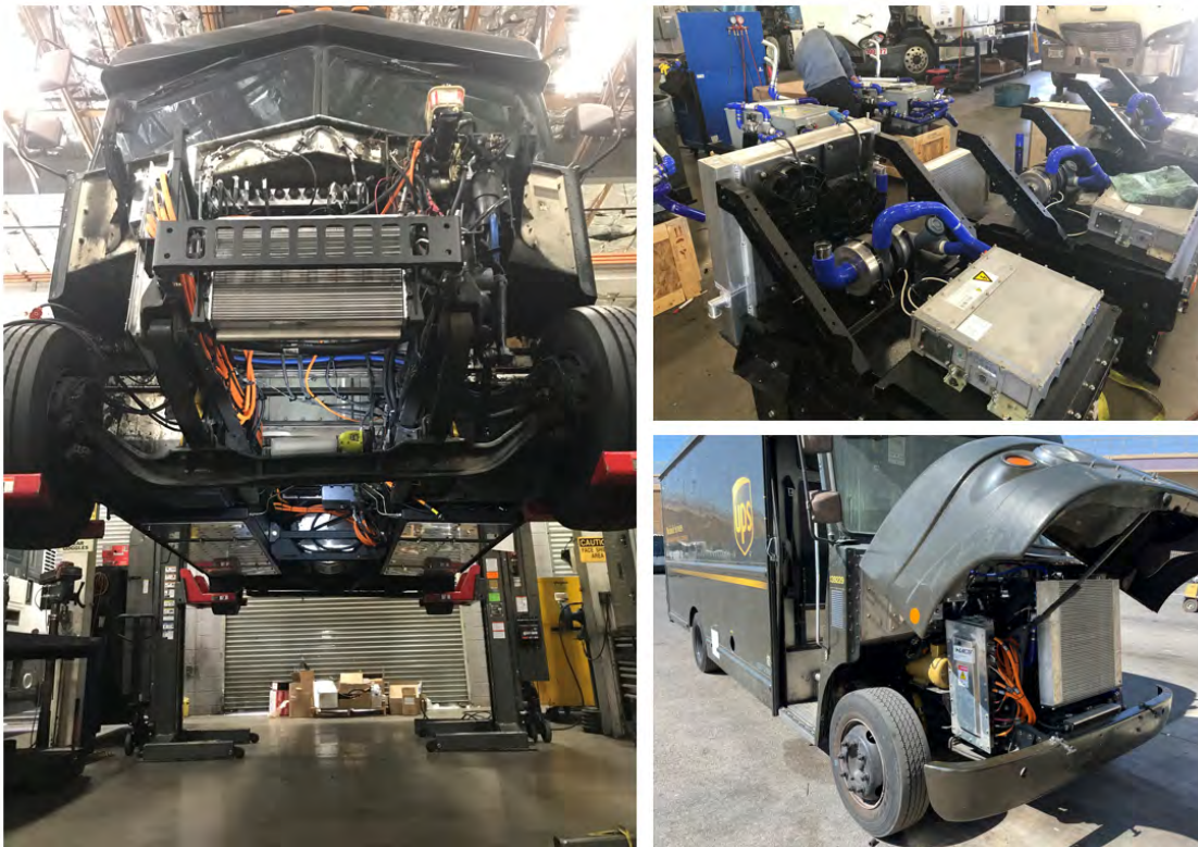
Figure 5: Phase 2 FCEV Repower Kit Assembly
