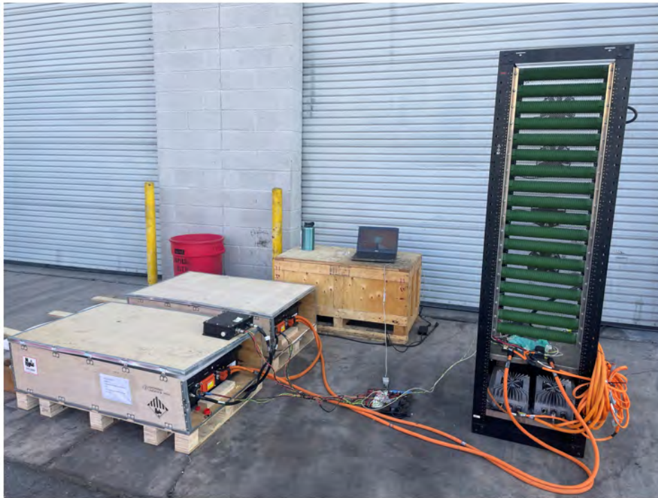
Figure 8: ESS Stationary Commissioning Cycle Fixture
