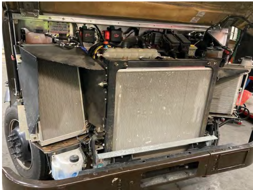
Figure 20: Front View Showing eAxle System, FC, and Battery Condenser Radiators
