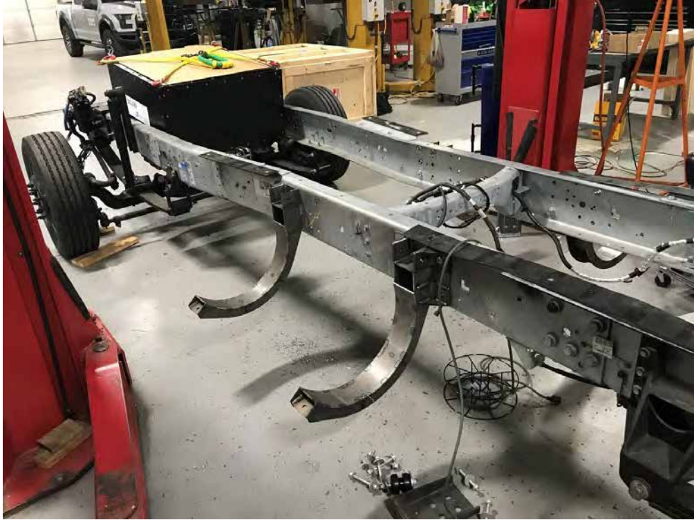
Figure 13: De-Contented F-59 Chassis Showing Fuel Cell and Hydrogen Tank Saddles (WIP)
