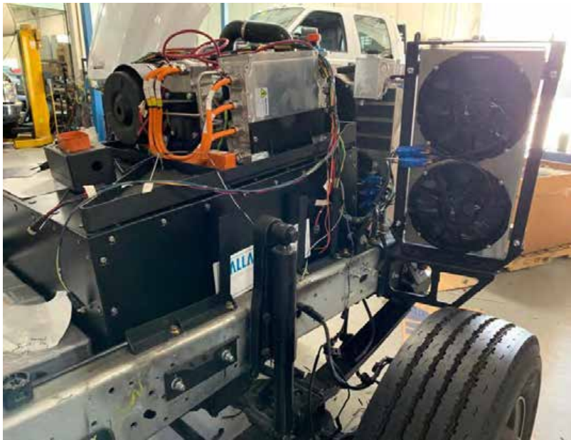
Figure 17: Fuel Cell with Air Handling System
