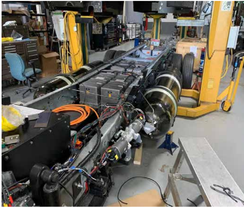
Figure 14: Hydrogen Tanks and Battery Modules on F-59 chassis
