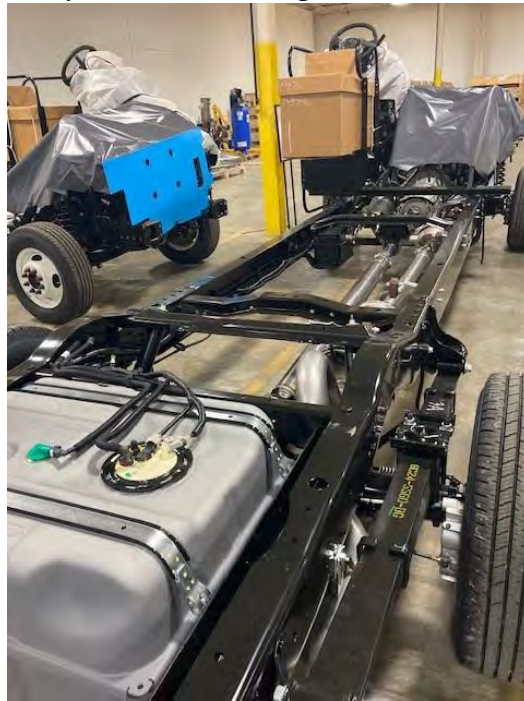
Figure 11: F-59 Stripped Chassis with Internal Combustion Engine components
