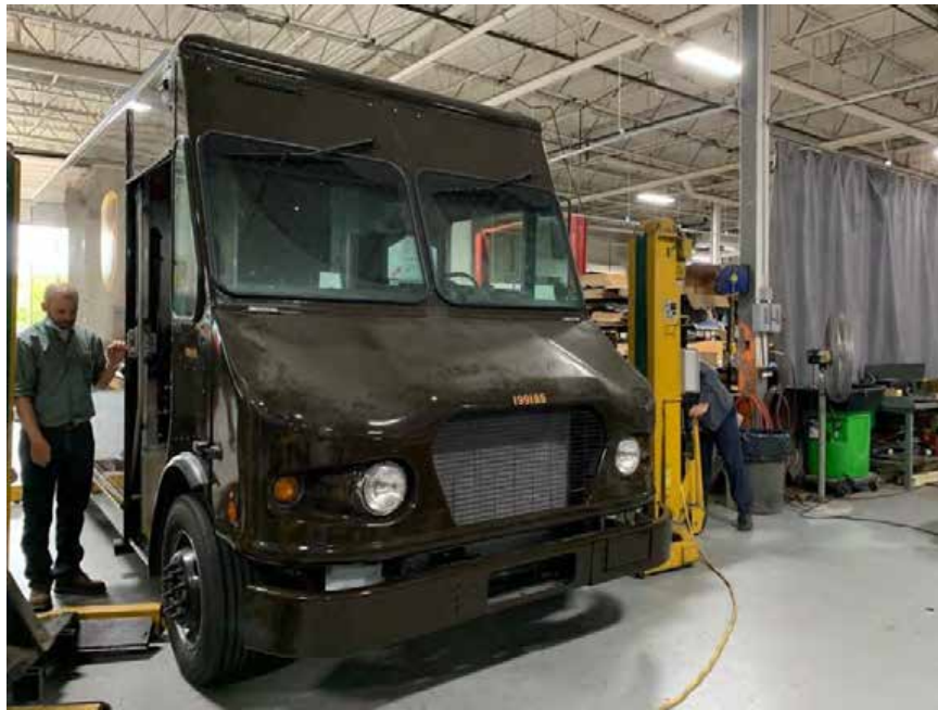
Figure 21: UPS P100 Truck Body Reinstalled on the Finished Chassis
