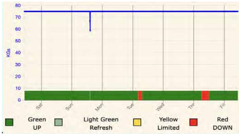
Figure 44: Iwatani Station Inventory and Uptime for May 18-24, 2024
