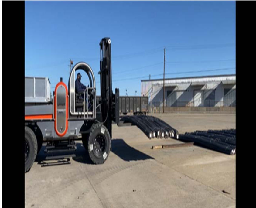
Note: Port operator hauling rebar at the Port Courtyard using the DANNAR MPS with the dump bed attachment.
