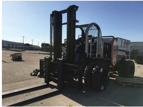
Unit with 30,000 lb forklift and dump (SN: MPD409919004)
