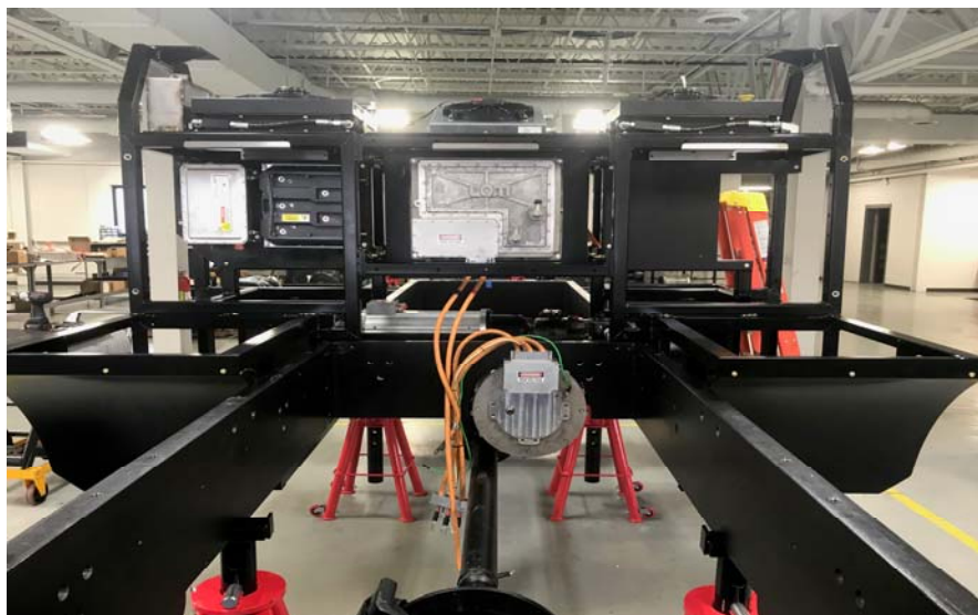
Note: Close up view of the black MPS chassis with additional framework for support equipment.
