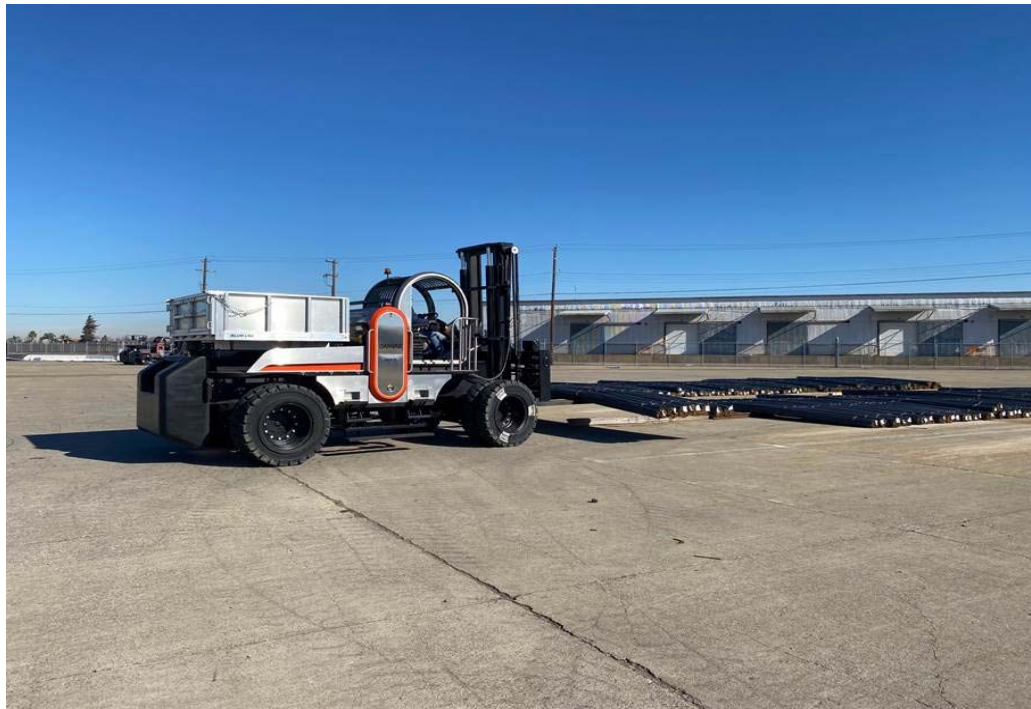
Note: Wide angle view of Port operator hauling rebar at the Port Courtyard using the DANNAR MPS with the dump bed attachment.
