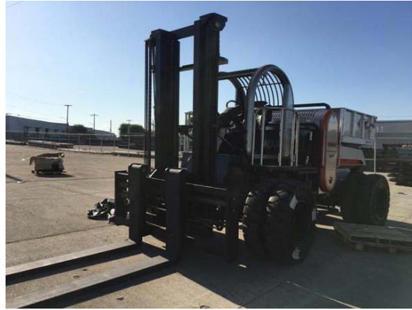
Electric Lift: 2019 DANNAR 4 MPS (LiO battery)
