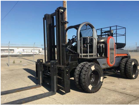
Unit with 30,000 lb forklift and manlift (SN: MPD413219003)
