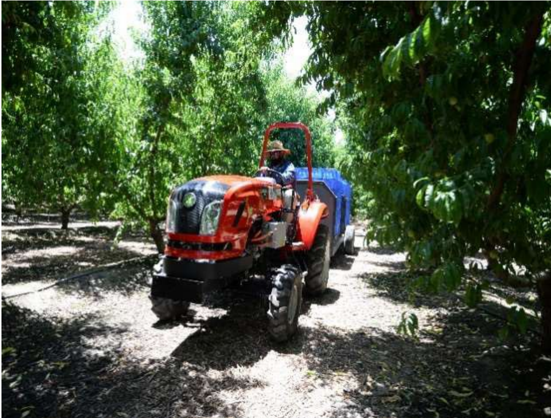
Figure #10: HummingbirdEV eTractor pulling bins in orchard at Demonstration Site, Moonlight Farms in Reedley, CA
