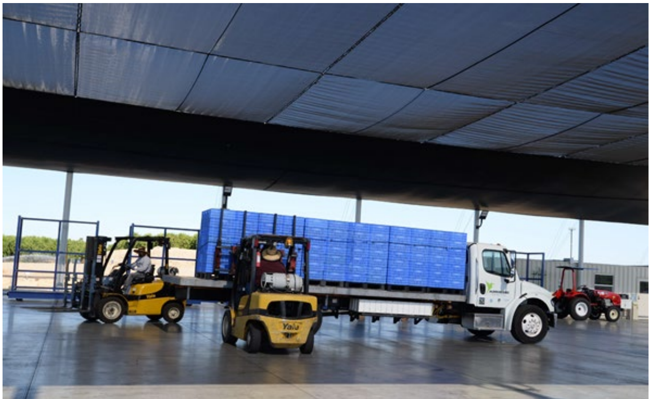
Figure #7: HummingbirdEV eTruck with End-User installed flatbed to move pallets of fruit at demonstration site, Moonlight Farms, in Reedley, CA.
