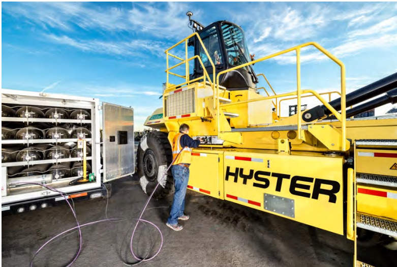
Figure 8: Fueling the Top Loader with GTM-1500
