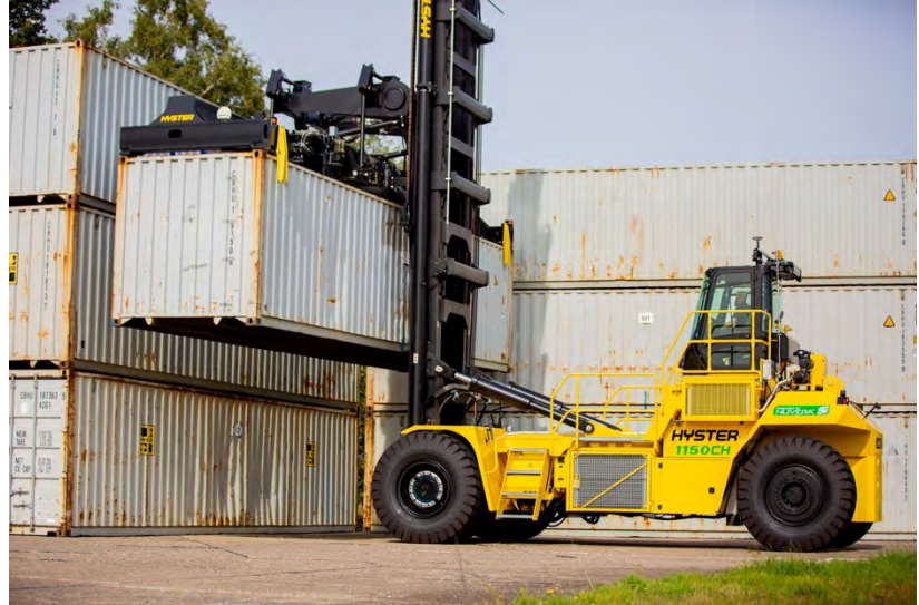
Figure 1: Top Loader Lifting Container
