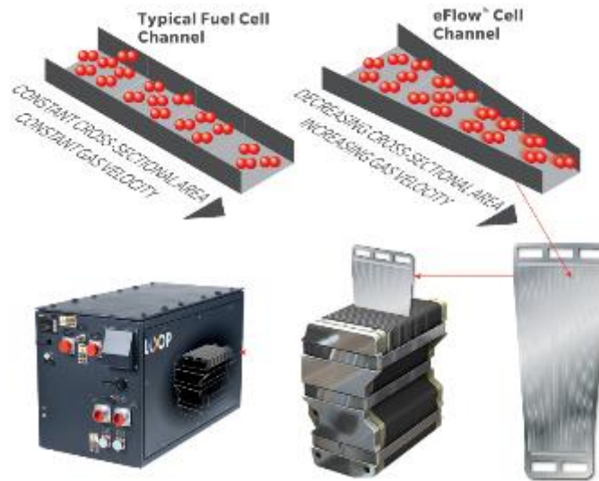
Figure 7 - Loop eFlow Cell Channel
