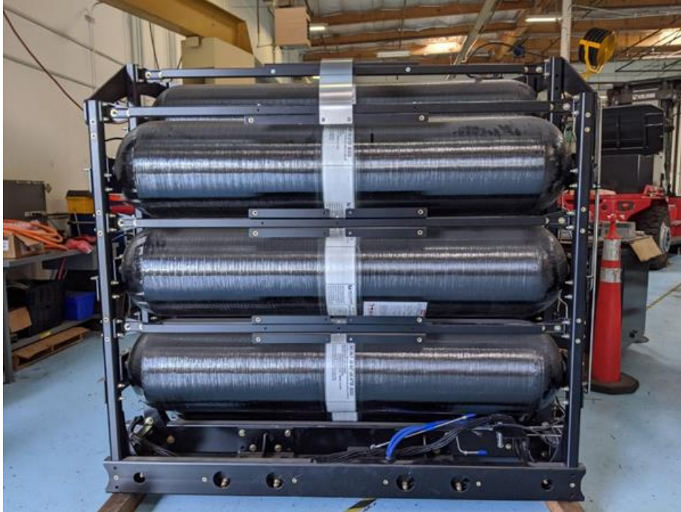
Figure 13 - Hydrogen storage ready for installation on FC6
