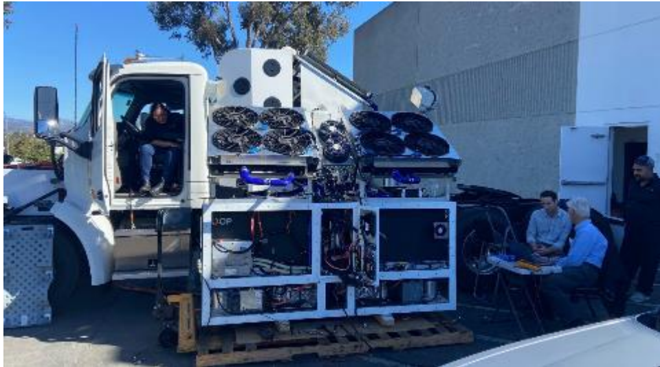
Figure 19 - Commissioning of fuel cells with FC7 (fuel cell modules are off-truck for accessibility)
