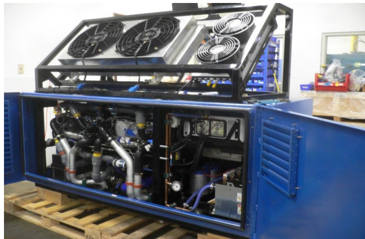
Figure 4 - Hydrogenics Fuel Cell System with Containment and Cooling Module
