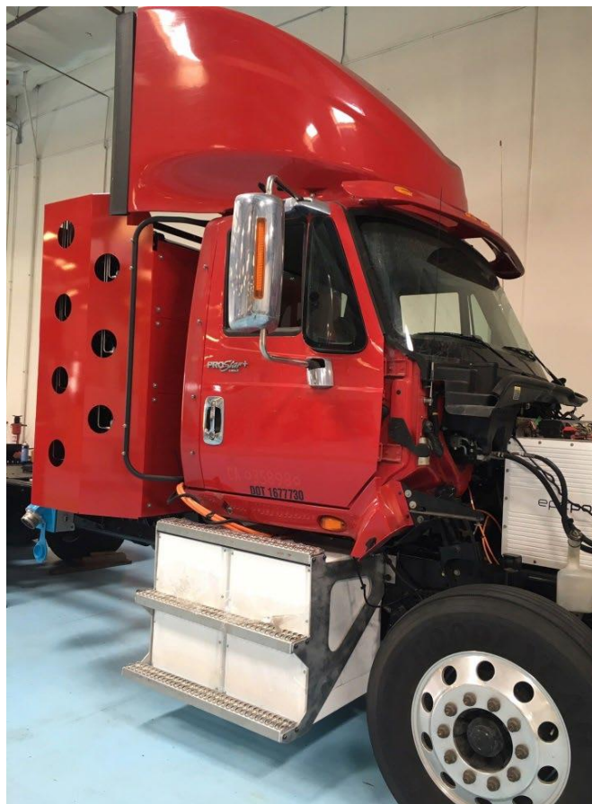
Figure 6 - Tanks shown mounted on the first Phase 1 truck
