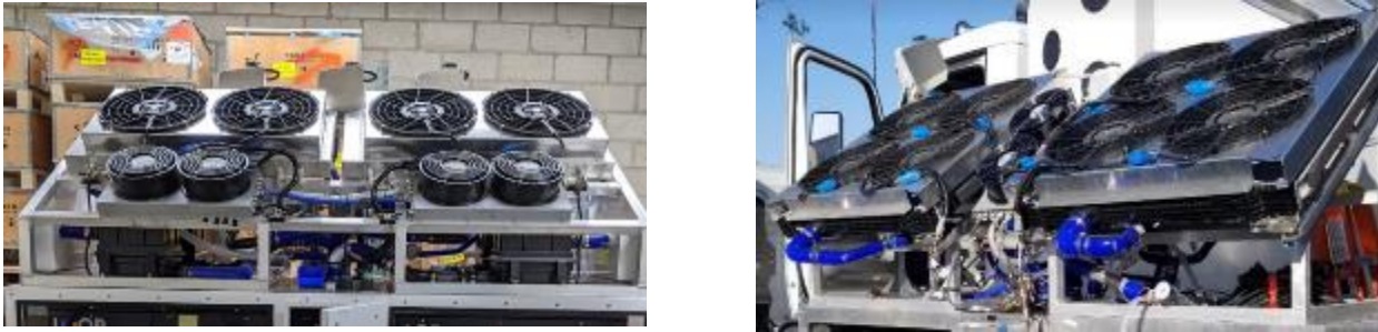
Figure 9 - Old cooling system (left) and redesigned cooling system (right)
