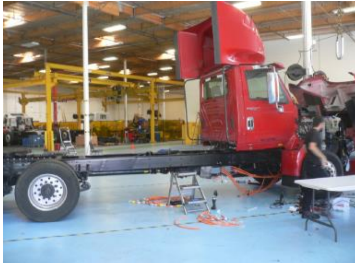
Figure 2 – Extended Frame Rails for Red Phase 1 FTFC truck Before Mounting, Tanks, Hydrogenics System and APU.
