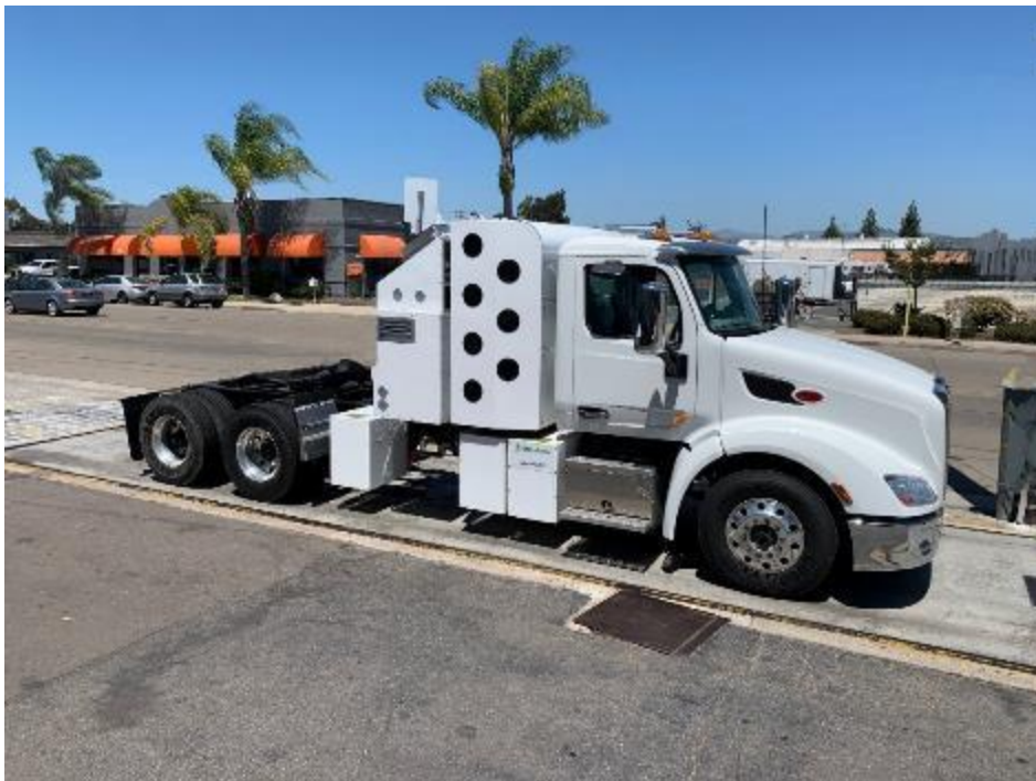
Figure 16 - FC6 truck on scales during on-road commissioning. The long wheelbase and additional equipment bring the curb weight to 23,300 lbs
