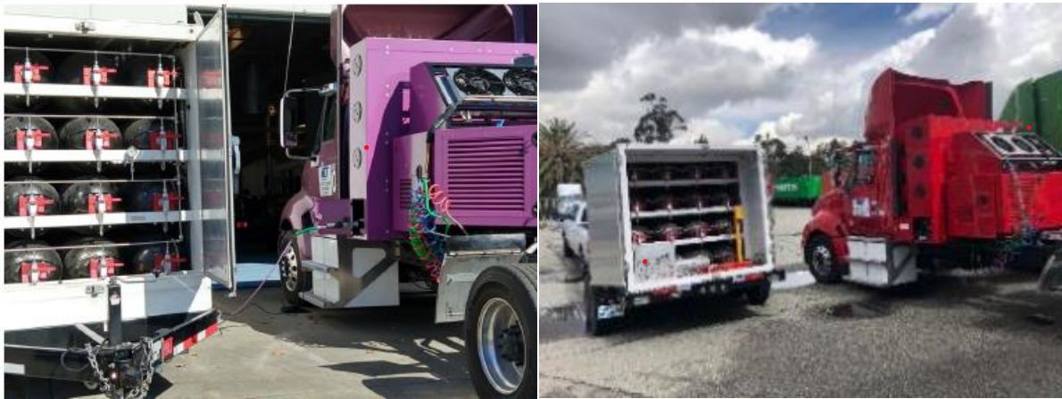
Figure 21 - IGX mobile fueler filling FC5 at TransPower (left) and FC3 at TTSI (right)
