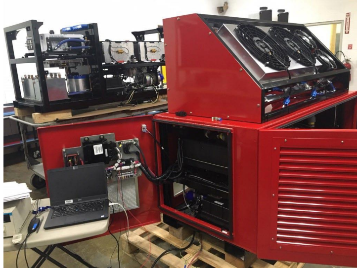
Figure 5 - Commissioning the first fuel cell system. The partially complete fuel cell system for truck FC3 is in the background. (March 2019).
