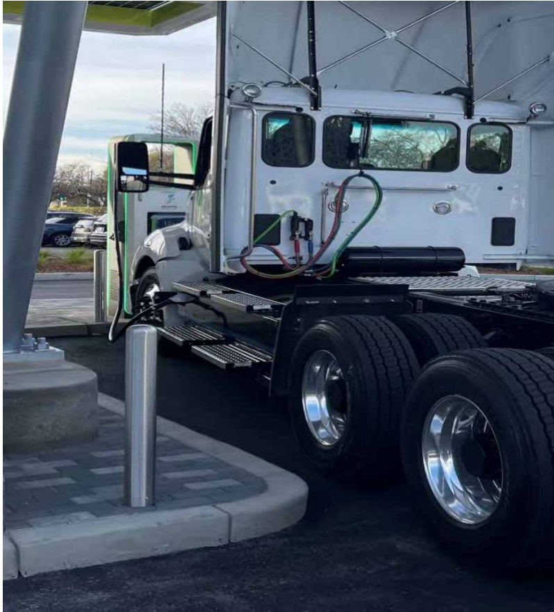
TransPower's Prototype Next Generation Drayage Truck Charging Using CCS-1 Charger in Sunnyvale, California
