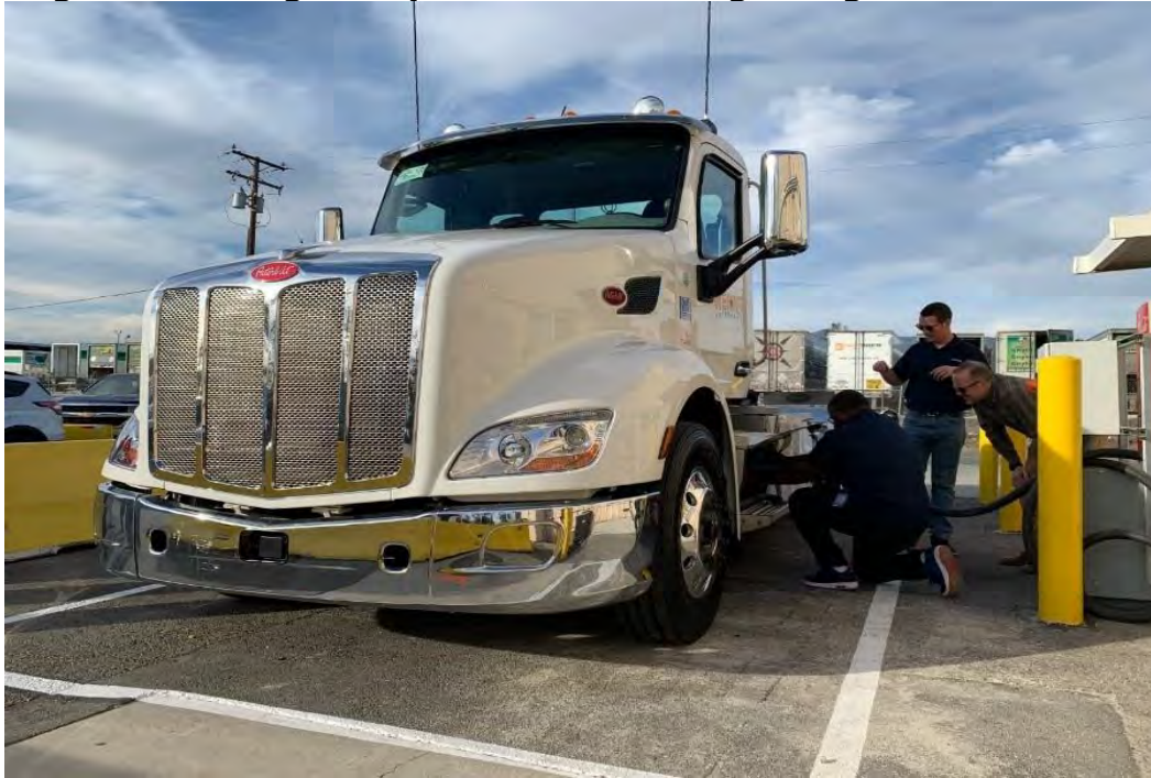
Figure 23: Image of Operator Connecting Charge Cable to GGRF ZEDT Truck
