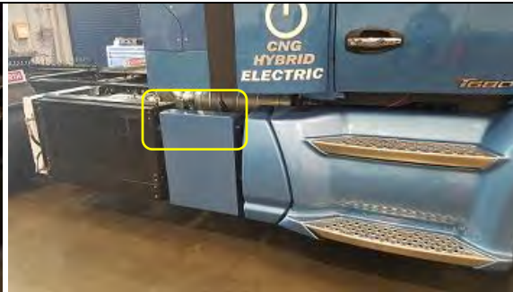
Figure 19: The LVPD box is located behind the side panel
