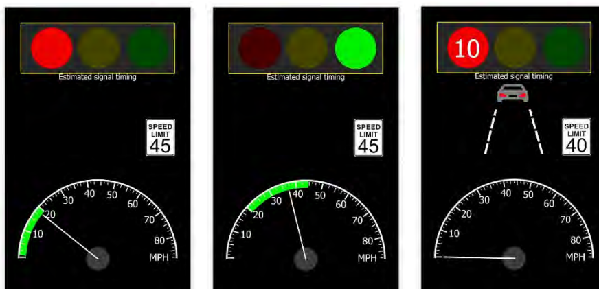
User interface of Eco-Drive indicating status of traffic signal, recommended range of driving speed, presence of preceding vehicle, and road speed limit
