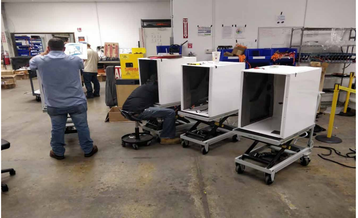
Figure 4: Redesigned Battery Electric Energy Storage System
