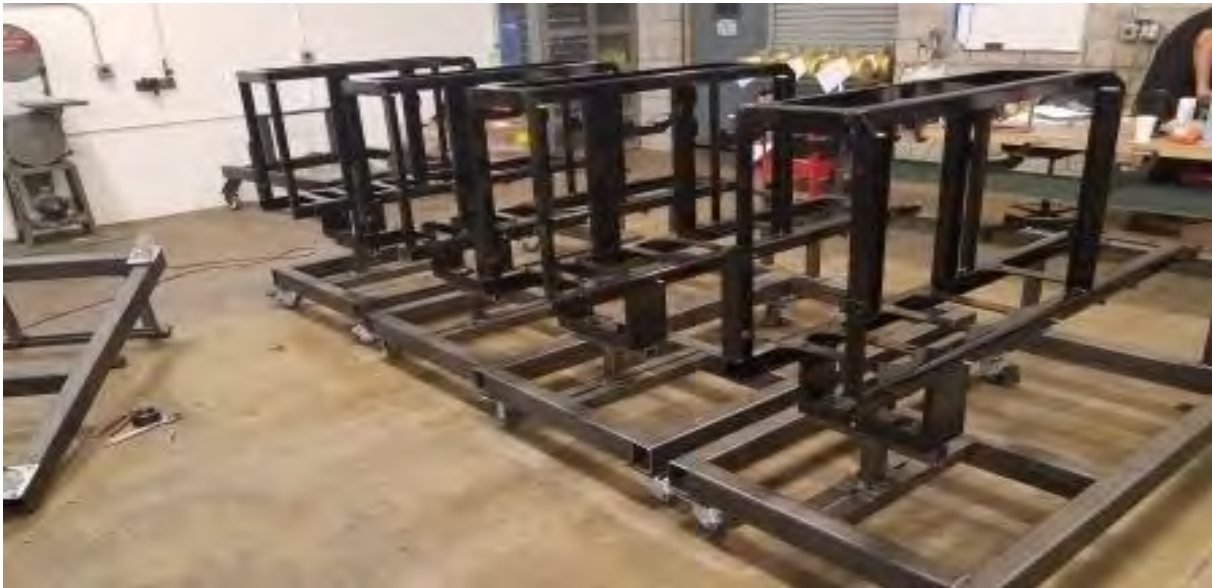
Figure 17: PCAS structures and Heavy-Duty MDS assemblies prior to integration into chassis
