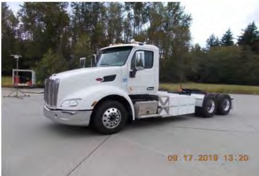
A Peterbilt Model 579 truck 8 ESS strings installed, 4 on each frame rail
