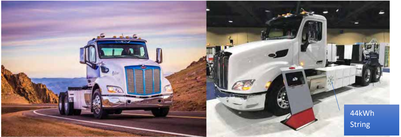
Two pictures, first of the TransPower NMC powered Peterbilt 579 tractor climbing Pikes Peak in CO and one of another 579EV staged at trade show. Credit: Peterbilt Inc
