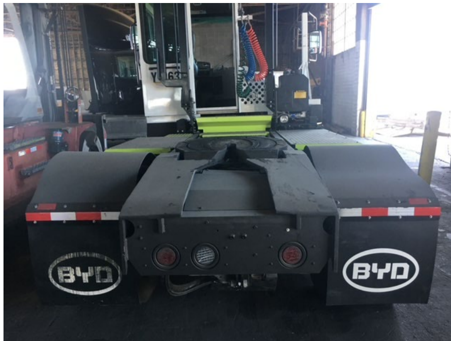
Figure 7: BYD Yard Tractor Fifth Wheel Retrofitted with Guides
