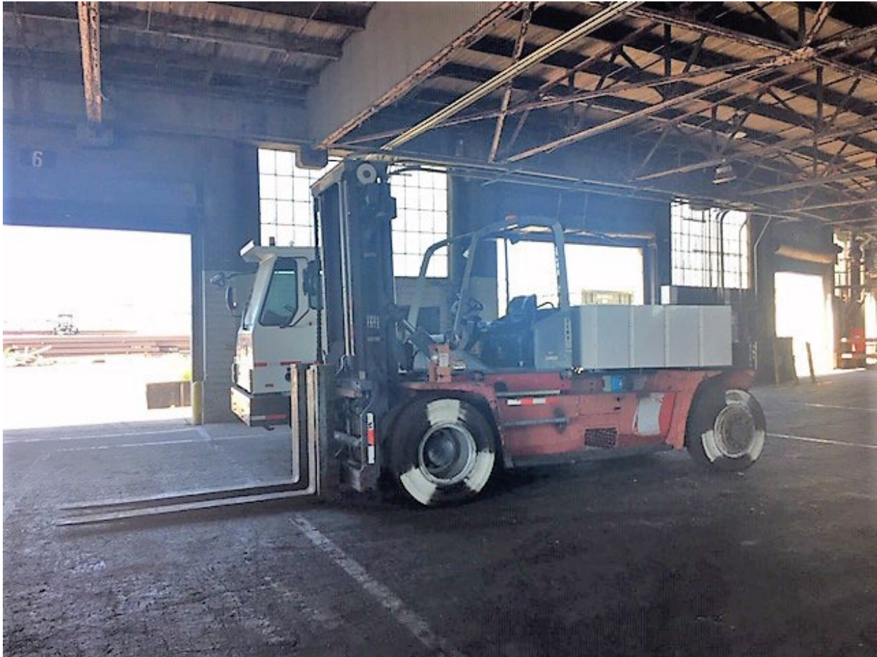
Figure 11: TransPower Repowered Battery-Electric Heavy-Duty Kalmar Forklift
