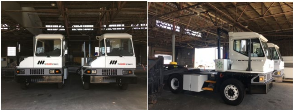
Figure 8: TransPower Battery-Electric-Repowered Kalmar T2 Yard Tractors
