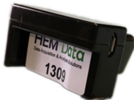
Figure 4-1: HEM DAWN OBD Mini Logger™ Used in this Project
